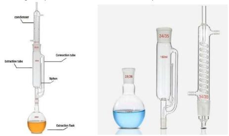
Liquid-solid extraction is to use the solvent for has large solubility of the required components and small solubility of impurities to achieve the purpose of extraction and separation.
